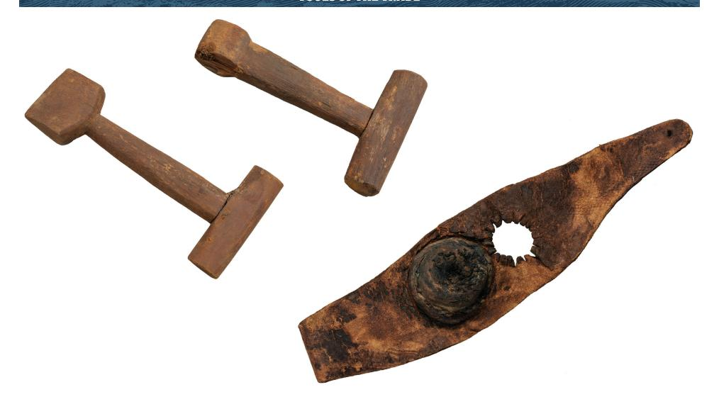
**SEAM RUBBER** Used to crease folded cloth and linen. (Left) SEWING PALM Protection for your palm from needles while sewing. (Right)
